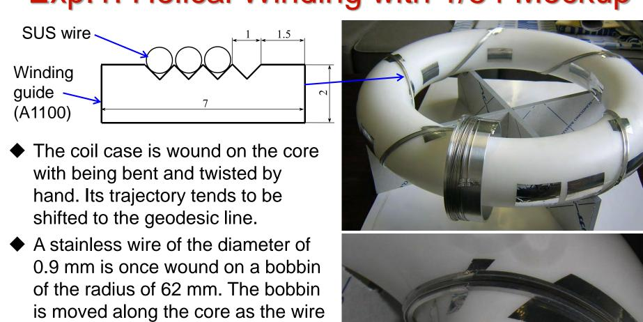
◆ By being pulled by hand, the wire is settled correctly in the grooves. This method is feasible in principle.
