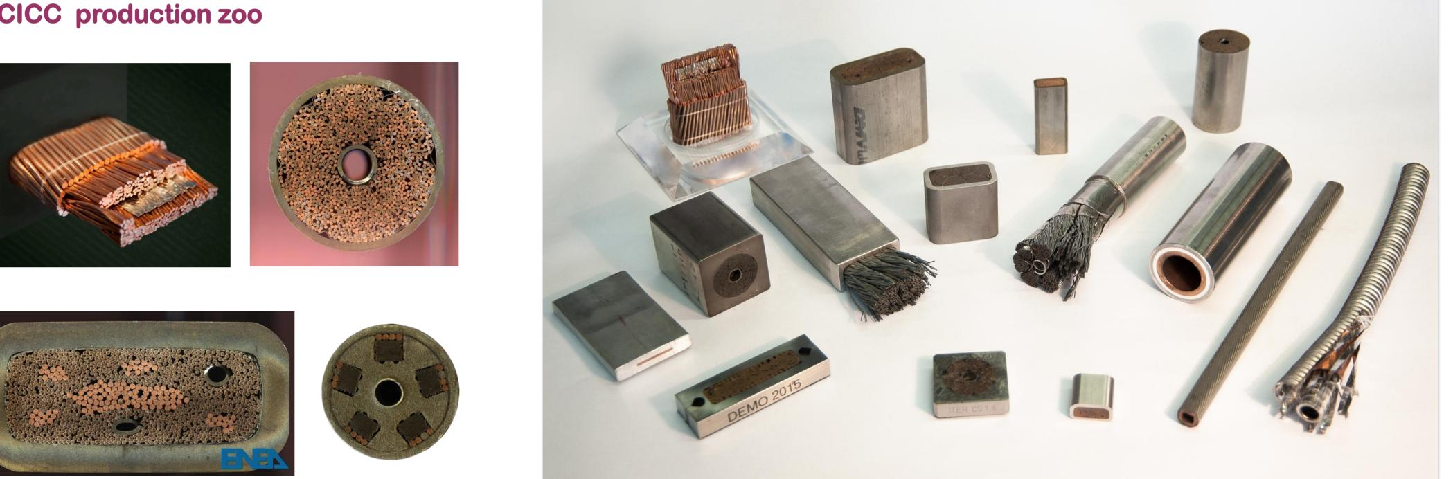
Impact of cabling process and cable layout on SC strands Possible defects may be caused to strands during cabling, in particular when very short Twist Pitch values are chosen. Measurements showed that only very large defects cause performance degradation. (R. Freda et al., "Performance Test of Superconducting Wires Subject to Heavy Deformations", http://hdl.handle.net/10840/6538)
