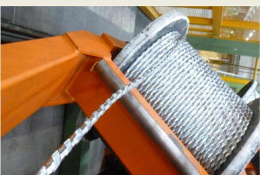
**JACKETING**: the flow of material within the conductor cross-section during the lamination process is influenced by the cable-jacket engagement.
