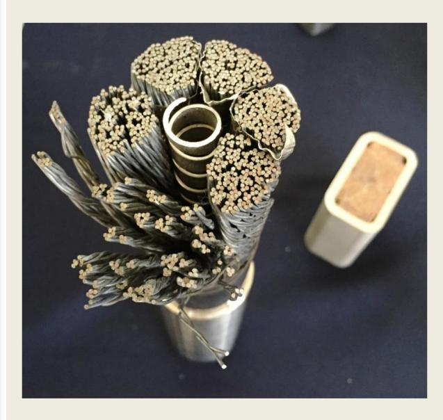
In principle, cabling SC is a standard process for any cabling company. BUT handling of SC wire requires adequate skills and attitude (mechanical stress limits; full traceability; relatively short unit lengths; management of leftovers; no joints and no breakages allowed; etc.).
