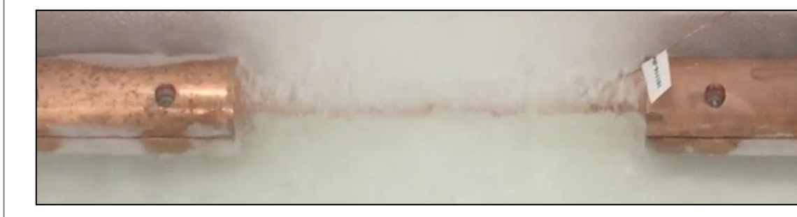
CORC® FCL wire during recovery
