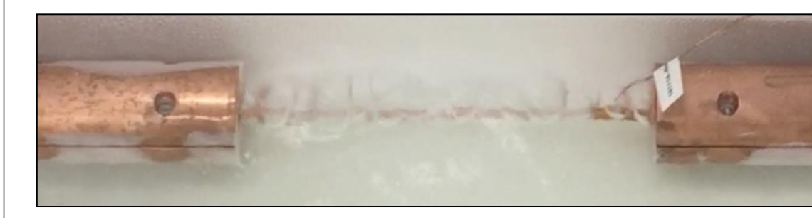
CORC® FCL wire at moment of fault
