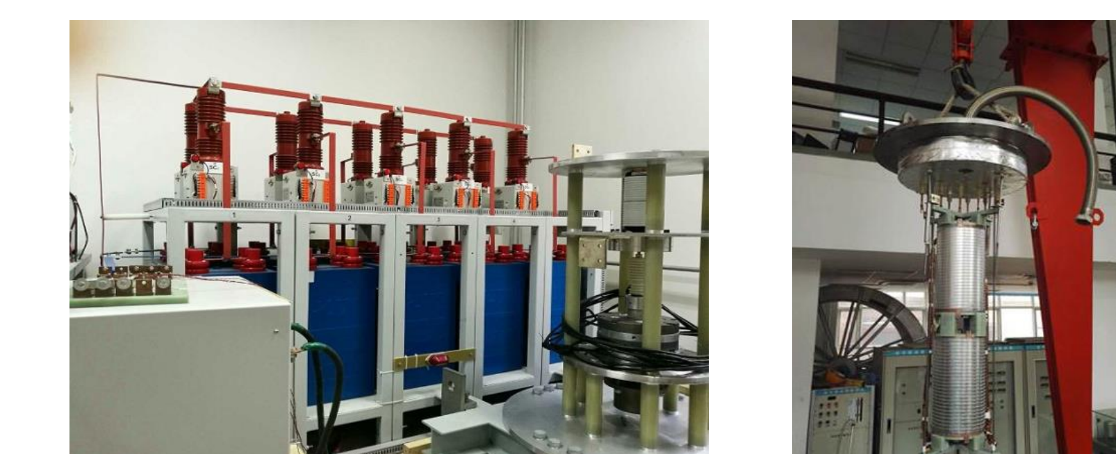
Fig. 10 Photograph of pulsed-dc power supply and FC-SFCL module.
