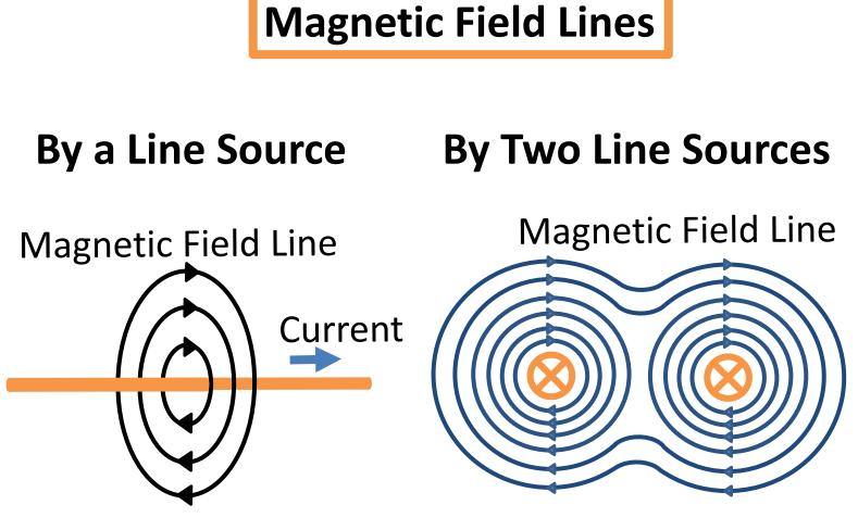
When there are multiple discrete line sources, the resultant magnetic field is a composition of the magnetic fields generated by individual line sources.
