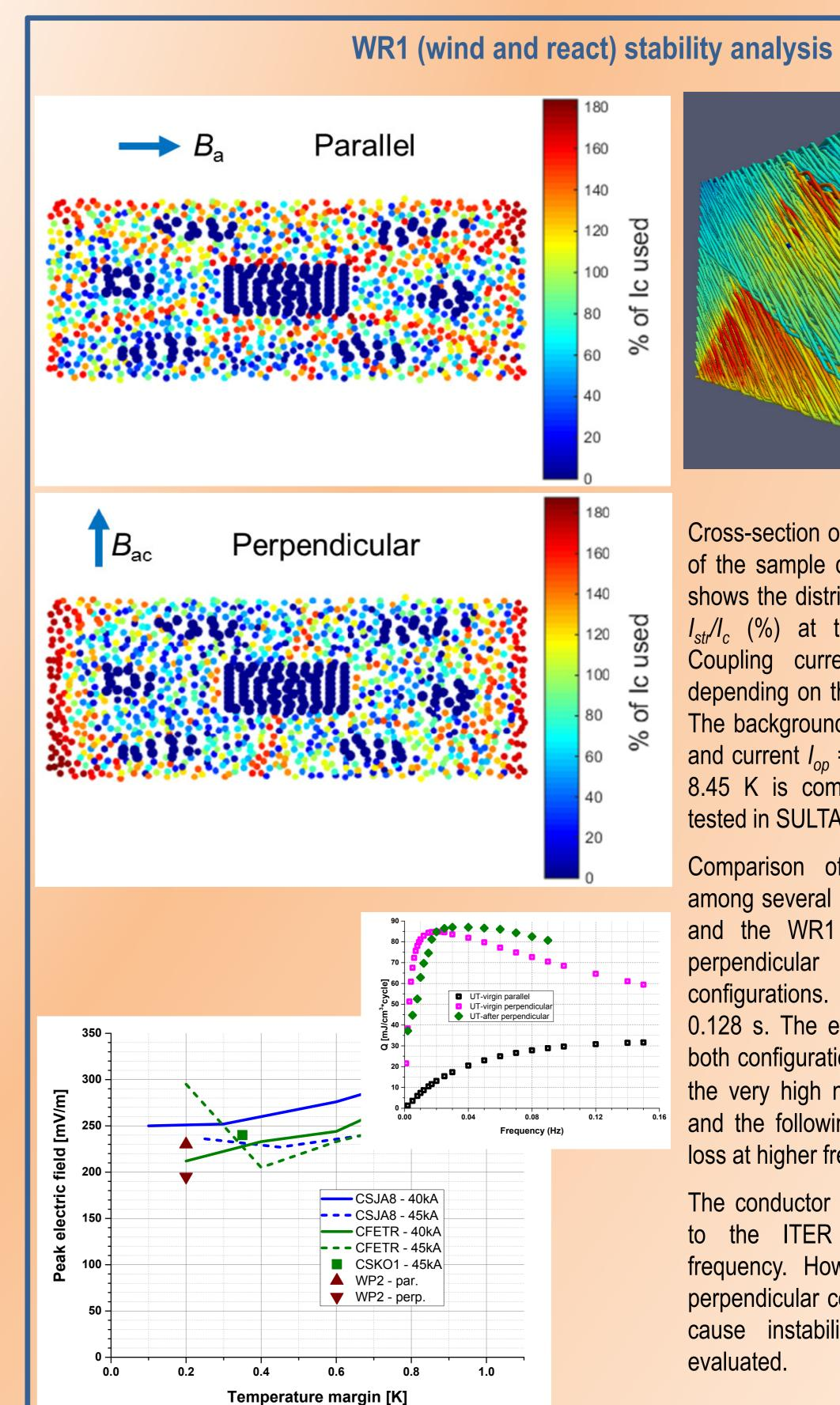
Cross-section of the conductor in the middle of the sample during stability test. The plot shows the distribution of the current as ratio  $I_{str}/I_c$  (%) at the maximum peak power. Coupling currents follow different paths depending on the magnetic field orientation. The background magnetic field  $B_{dc} = 11.8$  T and current  $I_{op} = 80$  kA. The calculated  $T_{cs} = 8.45$  K is comparable with CS conductor tested in SULTAN facility.
