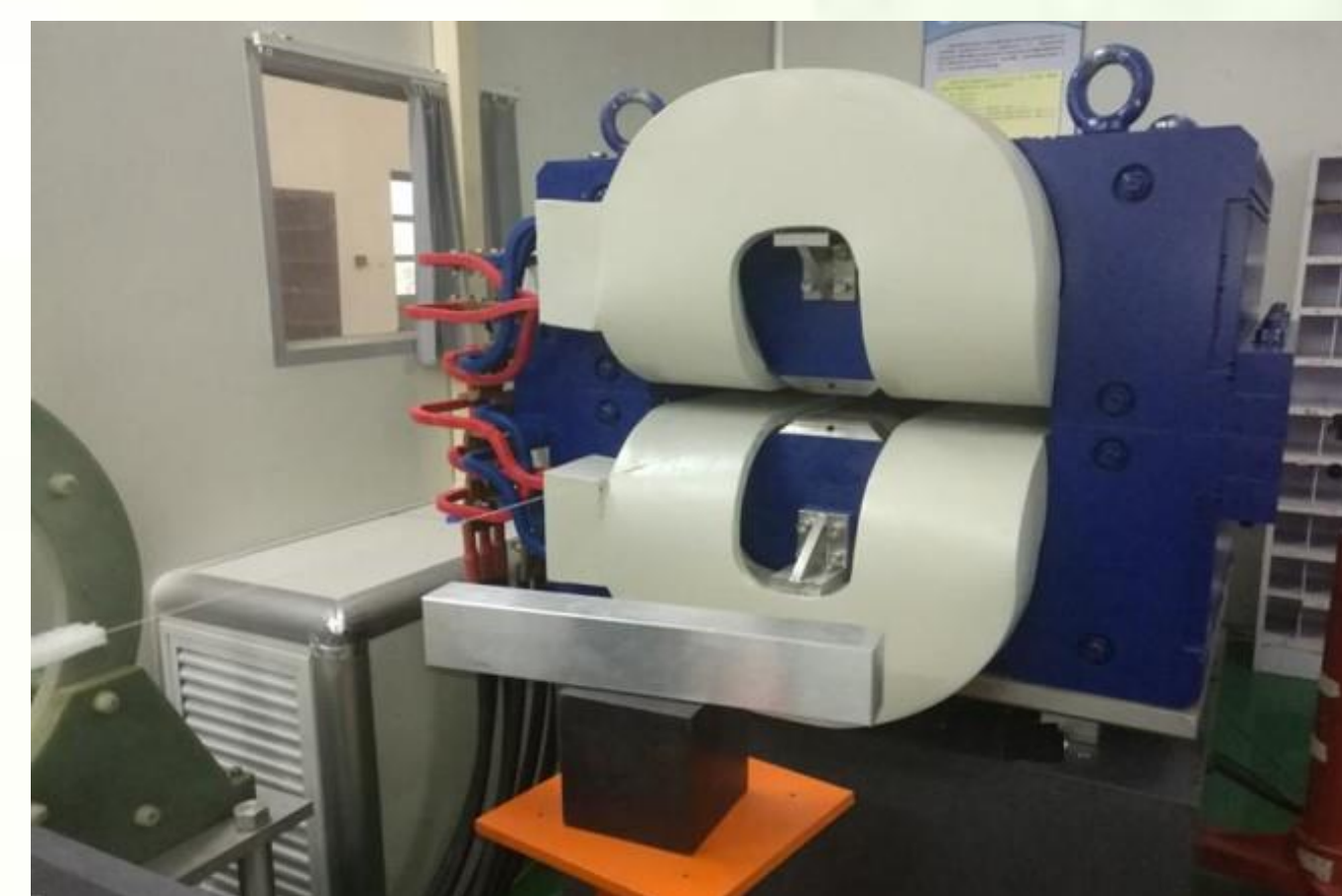
The magnet on a test bench in the magnetic measurement labory of SSRF
