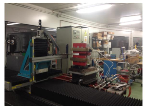
1) Calibration of the three hall probes with 5 probes RMN and new calibration method basec on modeling of the response of the probe to an external field.
