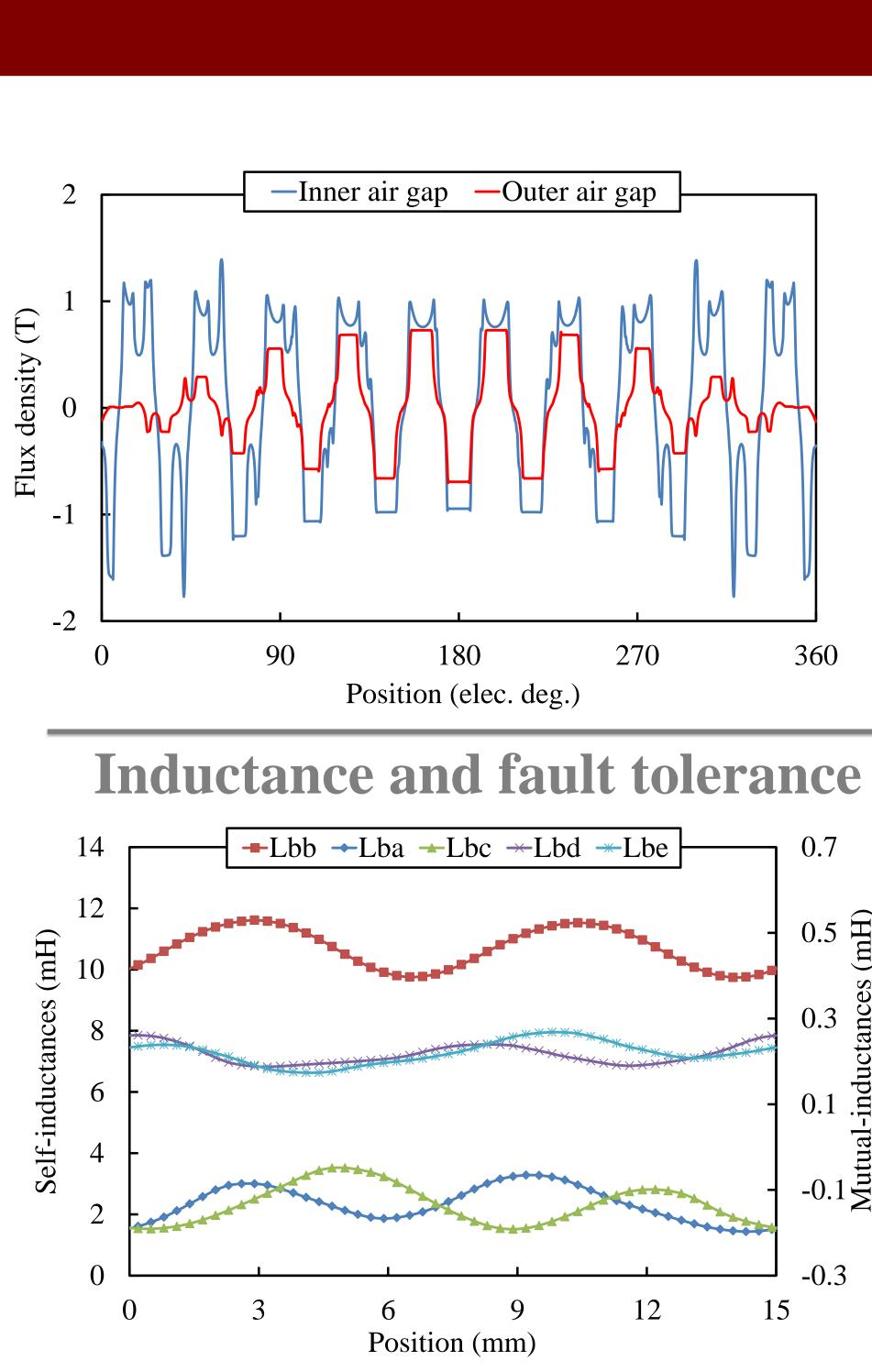
The ratio of mutual-inductance of self-inductance is only 2.1%. It further indicates that the magnetic fields of two adjacent phases are decoupled with each other. Therefore, the proposed motor can offer good fault-tolerant capability.
