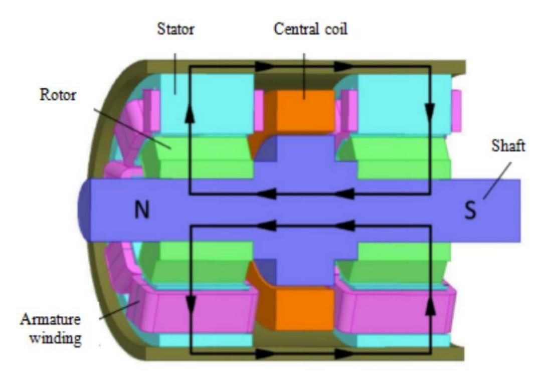
The armature winding produces the main magnetic field and the excitation coil generates an auxiliary magnetic field. The magnetic flux produced by windings and excitation coils travels through the guide and shaft to the rotors and then to the stators, and finally it forms a closed loop with the enclosure. According to the minimum reluctance principle, energized windings produce tangential stress in the air gap to drive the rotor rotate.
