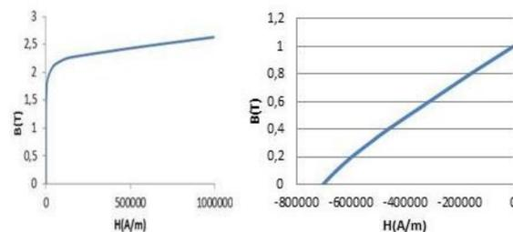
Fig. 5. Left; B-H curve of magnetic shielding. Right; magnetization of permanent magnet
