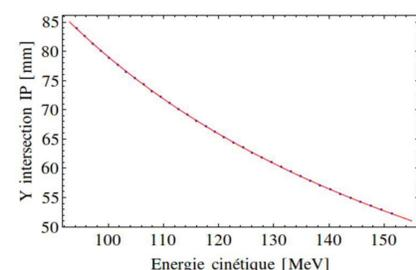
Fig. 16. Intersection, with rear IP, of high energy electron trajectories
