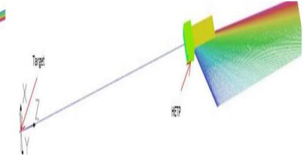
Fig. 13. Trajectories of high energy electrons deviated by HETP
