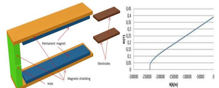
Fig. 9. Left; Geometry of half-LETP. Right; magnetization curve of LETP's permanent magnet.
