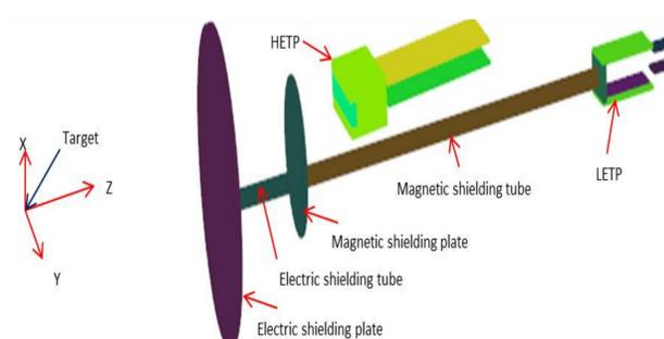
Fig. 8. Sketch of geometry of HETP and LETP and their magnetic shielding.
