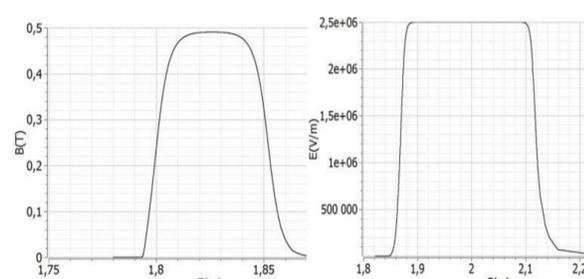
Fig. 7. Left; Evolution of magnetic field along the magnet's axis. Right; evolution of electric field along the magnet's axis
