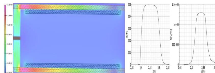
Fig. 10. Field map (in Tesla) on a vertical median plane XZ parallel to the beam's axis.
