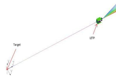
Fig. 14. Trajectories of low energy protons deflected by LETP
