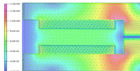
Fig. 6. Field map (in Tesla) on a vertical median plane XZ parallel to the emitted particle direction.
