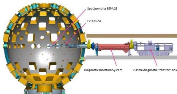
Fig. 1. Presentation of SEPAGE diagnostic during shot position
