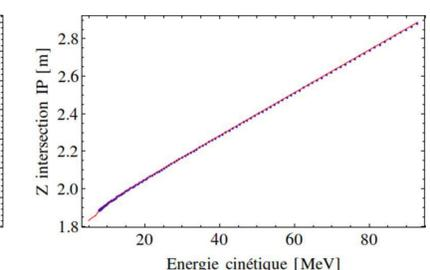
Fig. 17. Intersection, with lateral IP, of high energy electron trajectories
