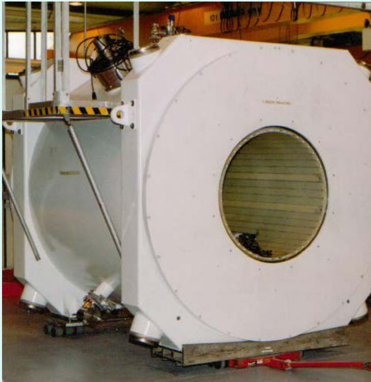
1 st generation 1.5T Active Shield
