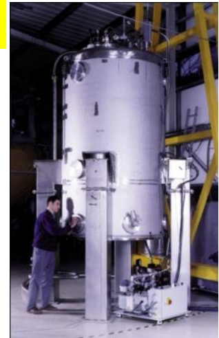
Stored energy of a 22 Tesla (950 MHz) 21 MJ
