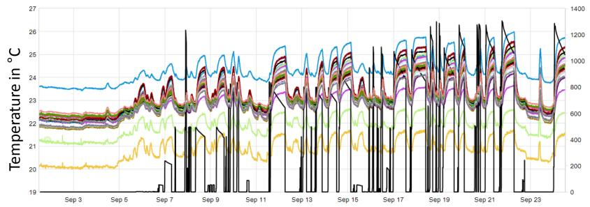
The temperature rise is dominated by changes in the air temperature in the tunnel.
