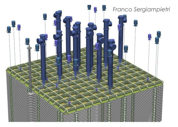
Integration of all the feedthroughs at the roof structure.
