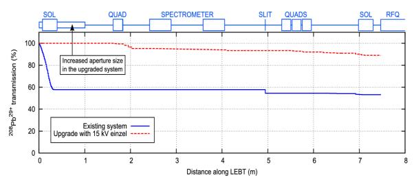
The best estimates from simulations is the 10-15% more intensity can be transported inside the acceptance of the RFQ.
