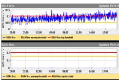
Detection boards suffer from meas. drift and very noisy signal due to high inductance and LEM hall probe sensor
