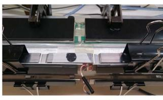
Inserts to leave 1mm thick circular ring for coolant
