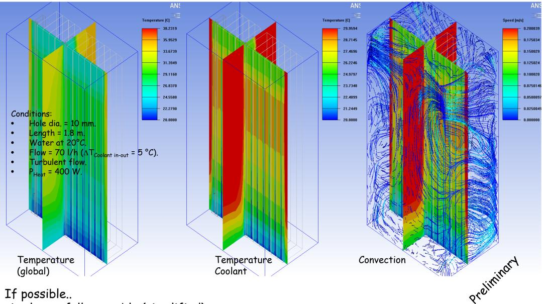
simulate a full assembly (simplified) including convection effect.
