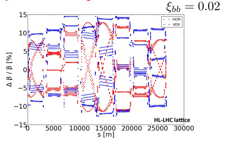
For beam-beam parameter of 0.03 this goes above 20% Synergy with HL-LHC studies T. Pieloni and R. Tomas Try to test experimentally local corrections in the LHC
