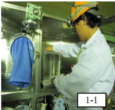
Figure 5 : Sealing box installation into the foil retrieving booth.
