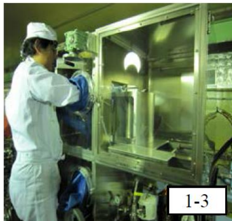
Figure 5 : Sealing box installation into the foil retrieving booth.
