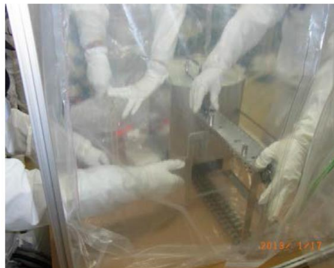
Figure9 : Retrieval of the radioactive foils from the holder storage rack.
