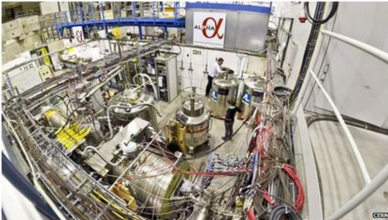
The Alpha experiment's antimatter chamber uses magnetic fields to sequester antihydrogen atoms
