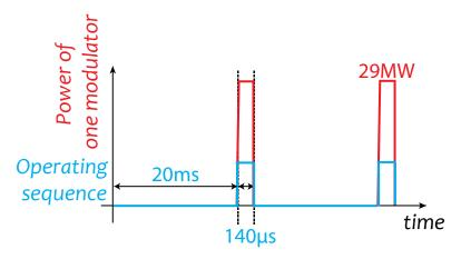
Absorbed AC power must be constant to stabilize distribution voltage!
