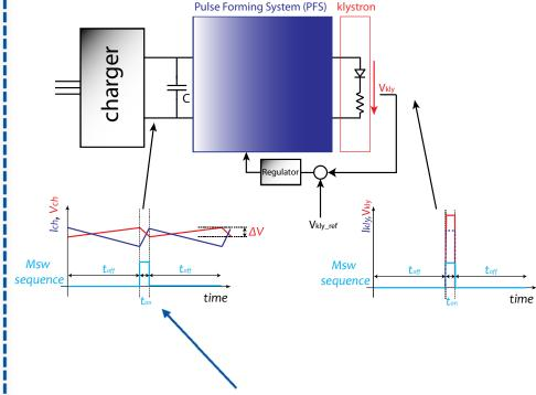
A solution consisting in high dynamics AFE to stabilize power (V\*I=const.)
