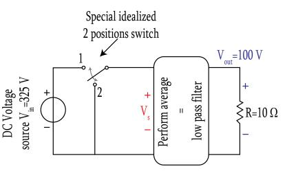
T<sub>s</sub>: switching period  $f_s = 1/T_s$ : switching frequency
