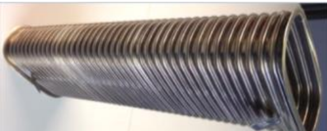
LiU-PSB : First prototype of BHZ chambers for new PSB H- injection (CZ-CH suppliers)
