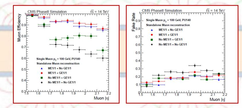
In all the cases, GE1/1 is able to recover the efficiency in the case of ME1/1 failure, even to introduce small improvement and reducing the fake rate.
