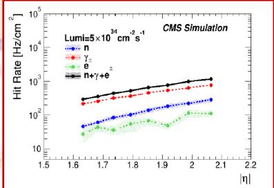
\* Photons and electrons produced from the neutron interactions in the material surrounding the enclosure that the GE1/1 chambers will be installed in 6
