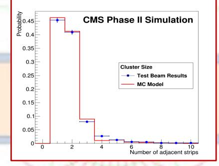
Comparison of the cluster size distribution obtained with simulations (red) and with the test beam measurements (blue)
