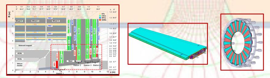
(Left): Schematic view, in the R-z plane, of one quadrant of the CMS detector, with the axis parallel to the beam (z) running horizontally and the radius (R) increasing upward. The interaction region is at the lower left corner. (Middle): A pair of GEM chambers form a superchamber (Right): Long and short chambers are combined with regards to the mechanical constraints.
