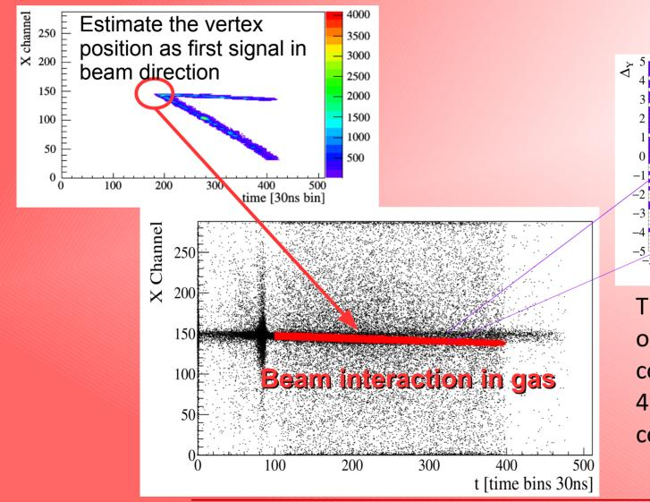
The vertexes are located on a region corresponding to the 4mm circular beam collimator
