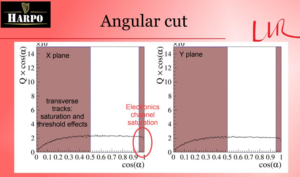
• The charge is normalised with regard to the track angle => independent of angle
