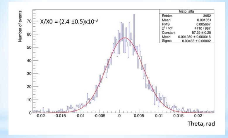
Measurements of spatial resolution of the triple-GEM detector (strip pitch 0.5 mm) Experimental results are corrected for multiple scattering and limited resolution of the tracking detectors
