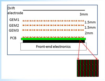
All measurements were performed with low-material triple-GEM detector for the photon tagging system of the DEUTRON facility at VEPP-3
