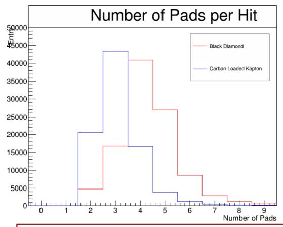
Number of pads that are fired when a charge cluster hits anode is 4.33 for BD and 3.13 for CLK.
