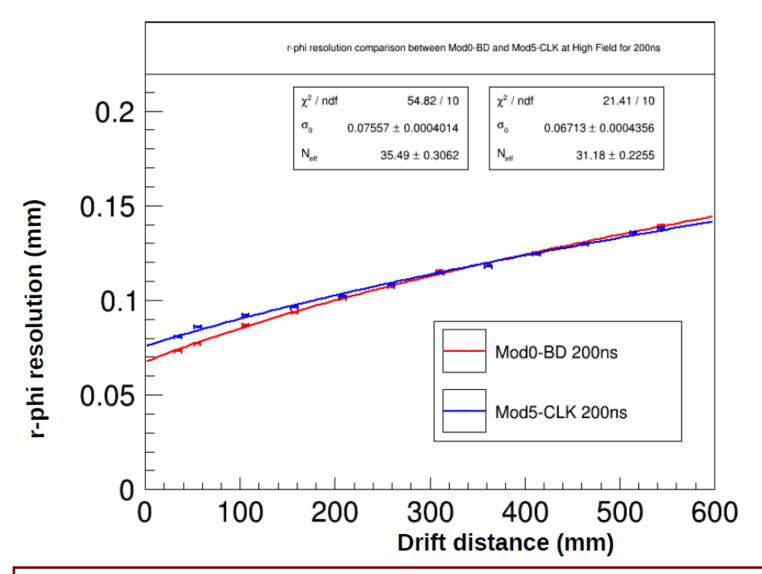
r-phi resolution comparison between a BD and a CLK (mod5) is shown. The two are very comparable.
