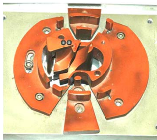
[inflector IBA Cyclone 30 cyclotron]
