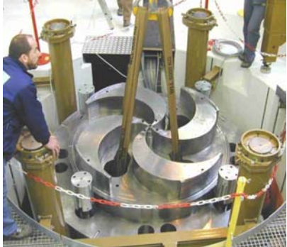
PSI/Varian comet: 250MeV sc. medical cyclotron
