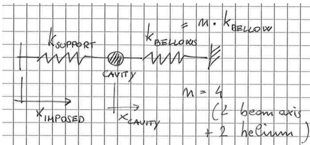
The lateral stiffness is not available on catalog (depends on the number of waves). The first  $k_b$  is an estimation from the angular stiffness, the second comes from an FE calculation (but not on the actual bellows).
