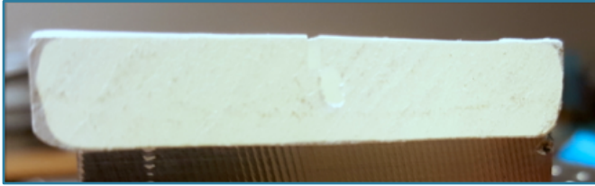
“Holey” extruded scintillator (5cm x 1cm)
