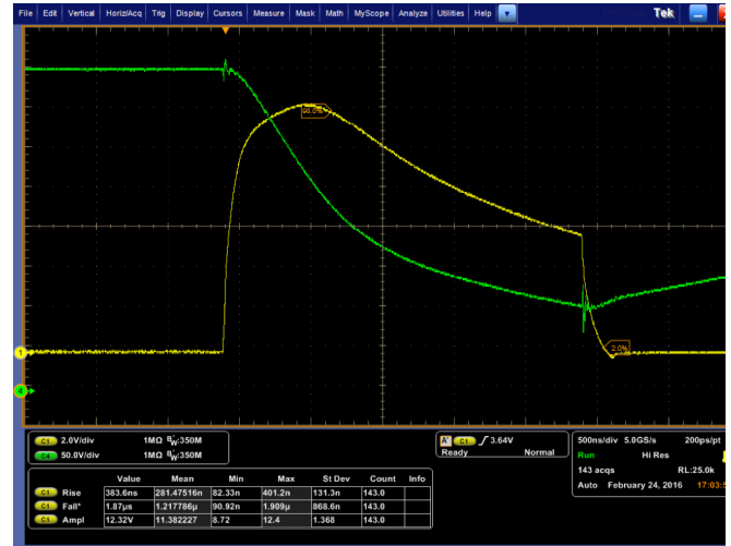
Fig. 11. Generator output short-circuited, with 400V input, first capacitor voltage (green) and output current (yellow): 50V/div, 8A/div, 200ns/div.
