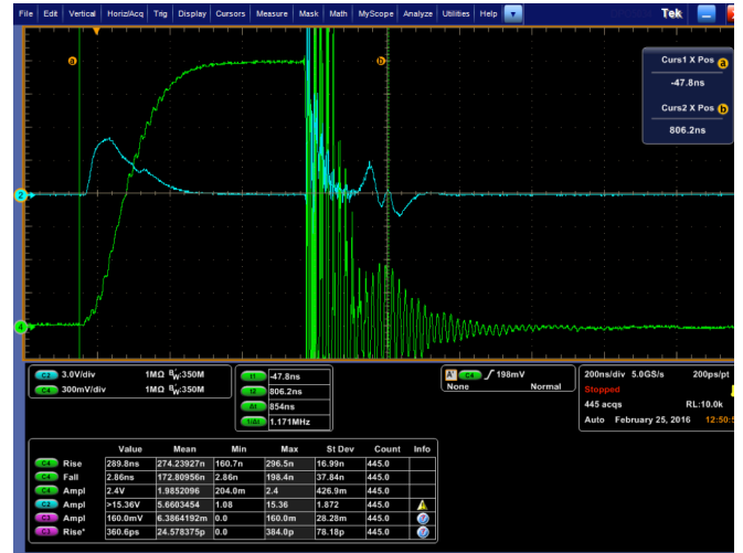
Fig. 14. Generator output connected to spark gap, 650pF, with 4.8kV output, pulse voltage (green) and current (blue): 600V/div, 5A/div, 200ns/div.
