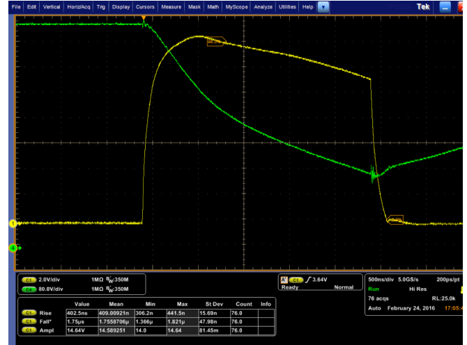
Fig. 12. Generator output short-circuited, with 700V input, first capacitor voltage (green) and output current (yellow): 80V/div, 8A/div, 500ns/div.
