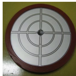
Fig. 1. Structure of a damaged thyristor valve with a specific gate structure designed to make the whole chip area ignited in a few microseconds [1].
