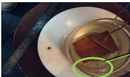
Fig. 11 Oil-pressboard samples with copper particles.
