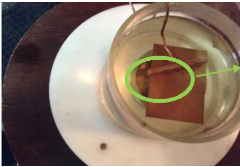
Fig. 9 Picture of copper particles at the center of the electrodes.
