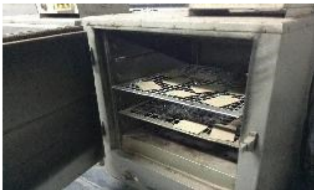
Fig. 2. Pressboards kept in hot air oven for drying
