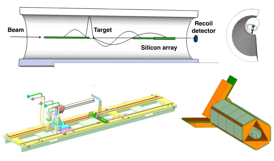
DSSDs with ASIC readout. x: 128 × 0.95 mm, y: 11 × 2 mm
