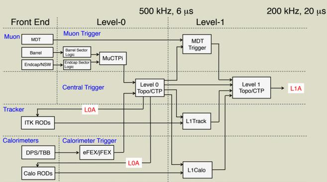
The proposed L0/L1 hardware trigger architecture for the Phase-II upgrade.
