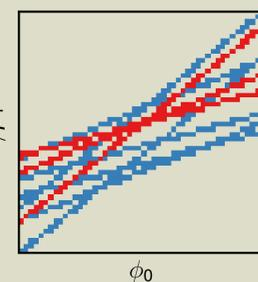
In this work, a single step of the Hough transform is applied to a  $\Delta\phi_0 = 0.2$  by  $\Delta\eta = 0.2$  RoI. The implemented accumulator is similar to a 2D histogram, but each bin holds information about which layers have been hit and a list of all hits in that bin.
