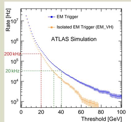
Trigger rates for pile-up 115 as a function of trigger threshold for isolated electron and tau triggers at the HL-LHC.
