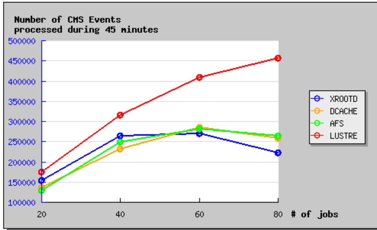
**Lustre definitively demonstrated itself as being the most efficient solution for this particular hardware configuration and the test program used.**
