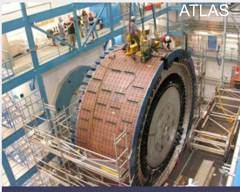
14 mm iron / 3 mm scint. sci. fibres, read out by phototubes
