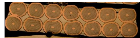
1 mm, 192 tubes PIT from Bruker EAS
