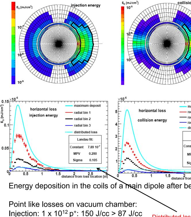
nergy deposition maxima in the old bore/beam screen.
