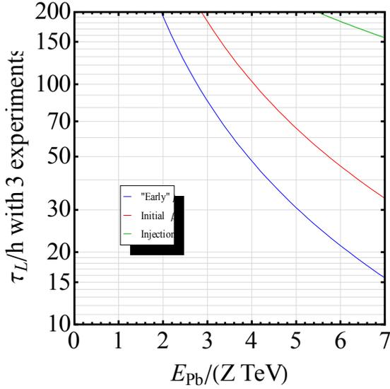
Figure 3: Initial luminosity decay times by burn-off alone for the three  $\beta^*$  variations in (3) at design emittance and full bunch intensity  $N_b = 7 \times 10^7$  in every one of the 62 bunches of the Early Beam structure.
