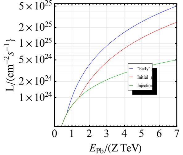
Figure 2: Potential peak Pb-Pb luminosity for the three  $\beta^*$  variations in (3) at design emittance and full bunch intensity  $N_b = 7 \times 10^7$  in every one of the 62 bunches of the Early Beam structure.
