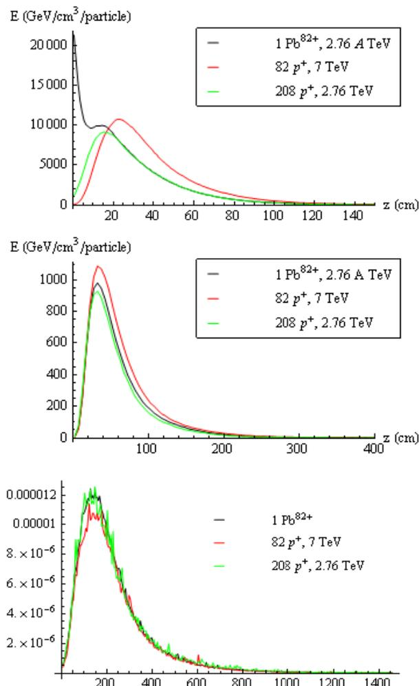
Figure 6: Levels of heat deposition resulting from a pencil beam of  $^{208}\text{Pb}^{82+}$  nuclei impinging on the beam screen at typical loss angles inside a dipole magnet, as simulated using FLUKA. From top to bottom, the plots show the hottest bin in the beam screen, the hottest bin in the superconducting coil and the energy deposition in a BLM outside the magnet cryostat (from R. Bruce).
