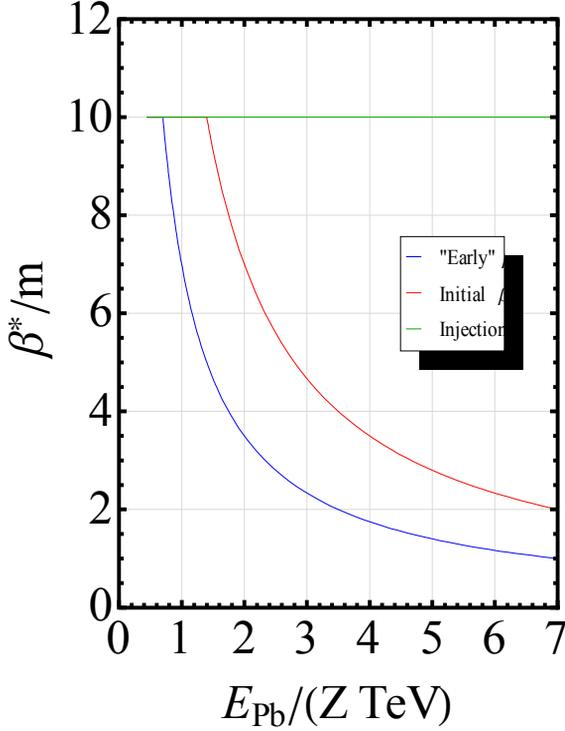
Figure 1 Energy dependence of the focusing function at the IP according to the three models of (2).
