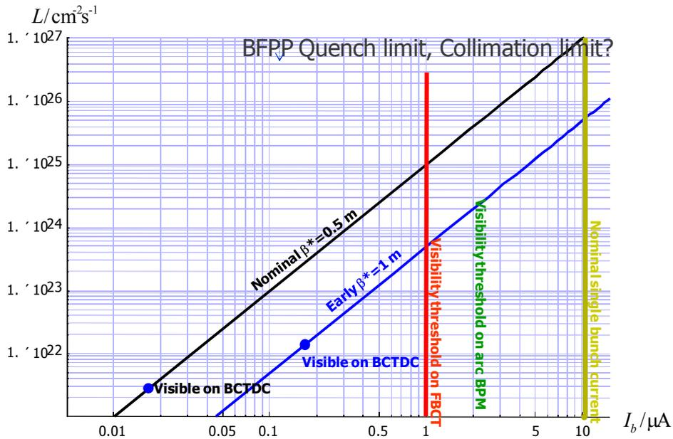
Figure 5: Variation of luminosity with single bunch current,  $I_b$ , for both the Early and Nominal ion schemes. Threshold of visibility on the FBCT and the arc BPMs are shown as vertical lines. Thresholds for the total current measured on the BCT DC are shown as points on the curves for the two schemes.
