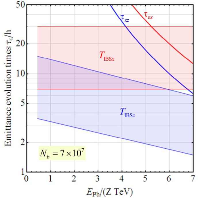
Figure 4: Time scales for emittance evolution by shrinkage due to radiation damping and IBS growth in transverse ( $\tau_{ex}$ ,  $T_{IBSx}$ ) and longitudinal ( $\tau_{ez}$ ,  $T_{IBSz}$ ) planes. A range of possible values for the IBS growth times is indicated depending on factors such as betatron coupling and the availability of controlled blow-up of longitudinal emittance using RF noise.
