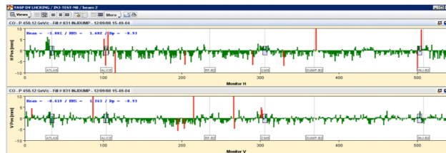
Figure 12: Best B2 closed-orbit as established on Friday 12th. The RMS orbit deviation excluding a few suspicious monitors is about 1.6 mm (horizontal) and 1.3 mm (vertical), compatible with the expected tolerance from beam dynamics. Faulty monitors (red) are disregarded for the RMS calculation.
