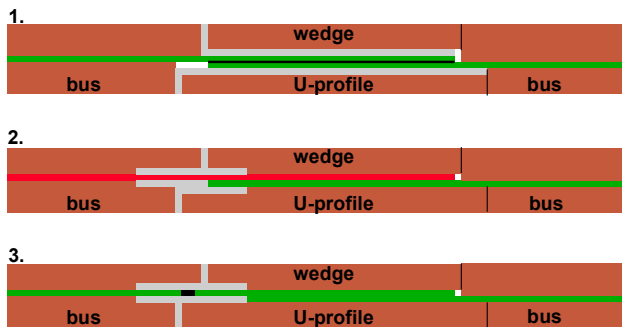
Figure 10: Three possible scenarios that could have been the origin of the fast thermal runaway during the incident.
