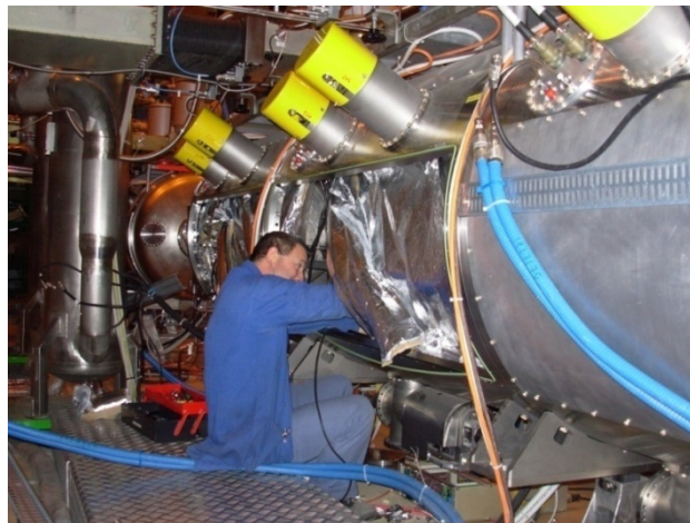
Figure 3: Replacing Tuner Cables in RUX45.
