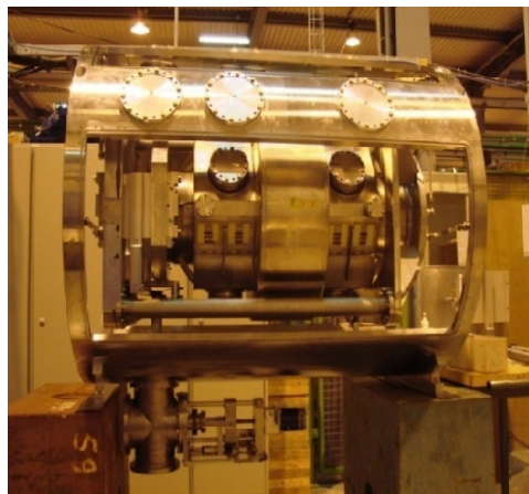
Figure 2: Open SC Cryostat Module, showing Helium Tank and Tuning Frame.
