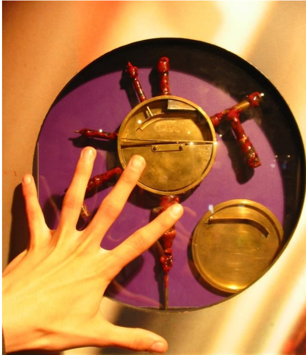
The first cyclotron (1930) D~11cm, E~1.1 MeV
