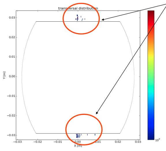
Vertical losses consistent from the aperture bottleneck measurements
