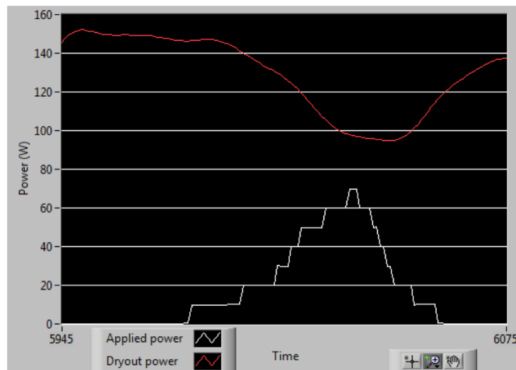
Figure 10: A Labview plot of showing, as a function of time, the power dissipated into a prototype microchannel substrate during stable running of the cooling circuitry (white graph). It also shows the maximum cooling power possible calculated from a real-time measurement of the mass-flow and knowledge of the latent heat of \text{CO}_2 . A maximum vapour quality of \sim 80\% is inferred.
