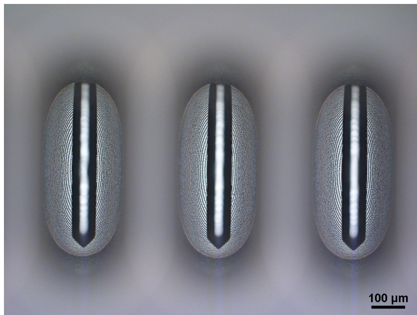
Figure 5: Photograph of a prototype showing the alignment of the DRIE-cut entrance slits (oval, in focus) and the beginning of the microchannel (elongated dark feature, out of focus).
