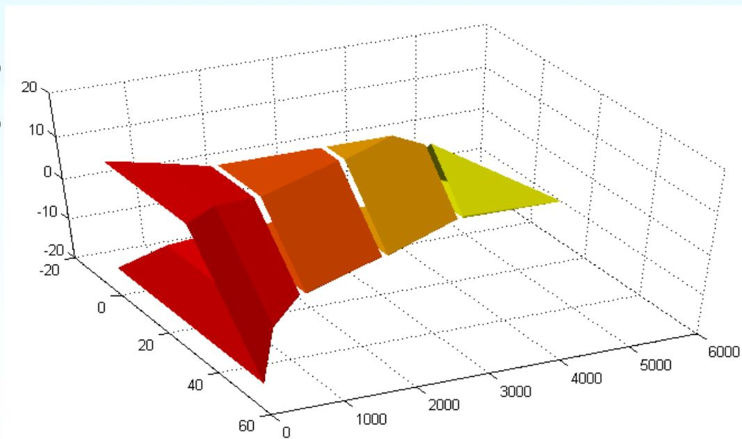
6 m length final absorber can absorb up to 170 kW of SR power
