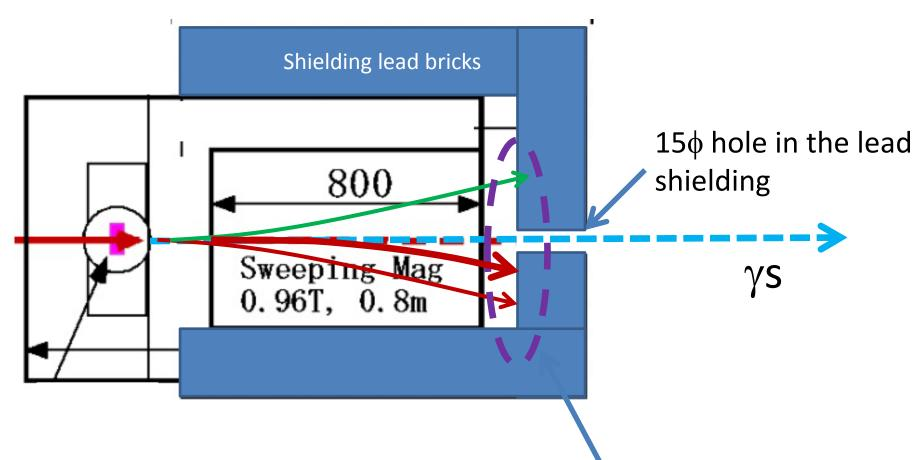
All charged particles are dumped here when the Sweeping magnet ON
