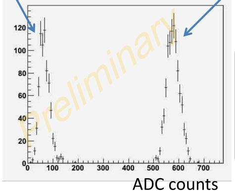
Signal is well separated from background even with thin converter
