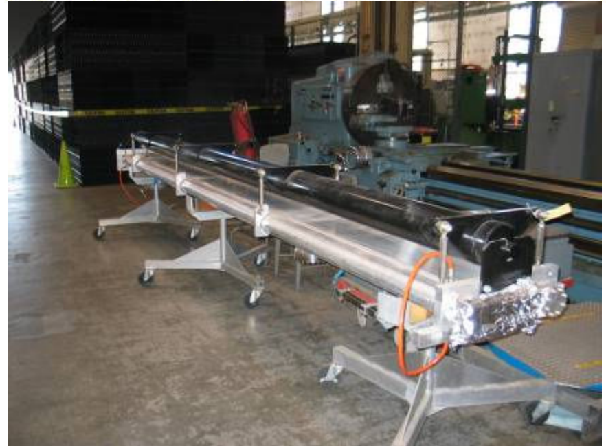
SLAC: PEP-II chamber analysis of TIN surface after 10 years
